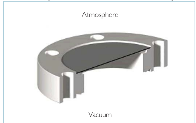
Cutaway of Standard UHV Be Window Assembly
