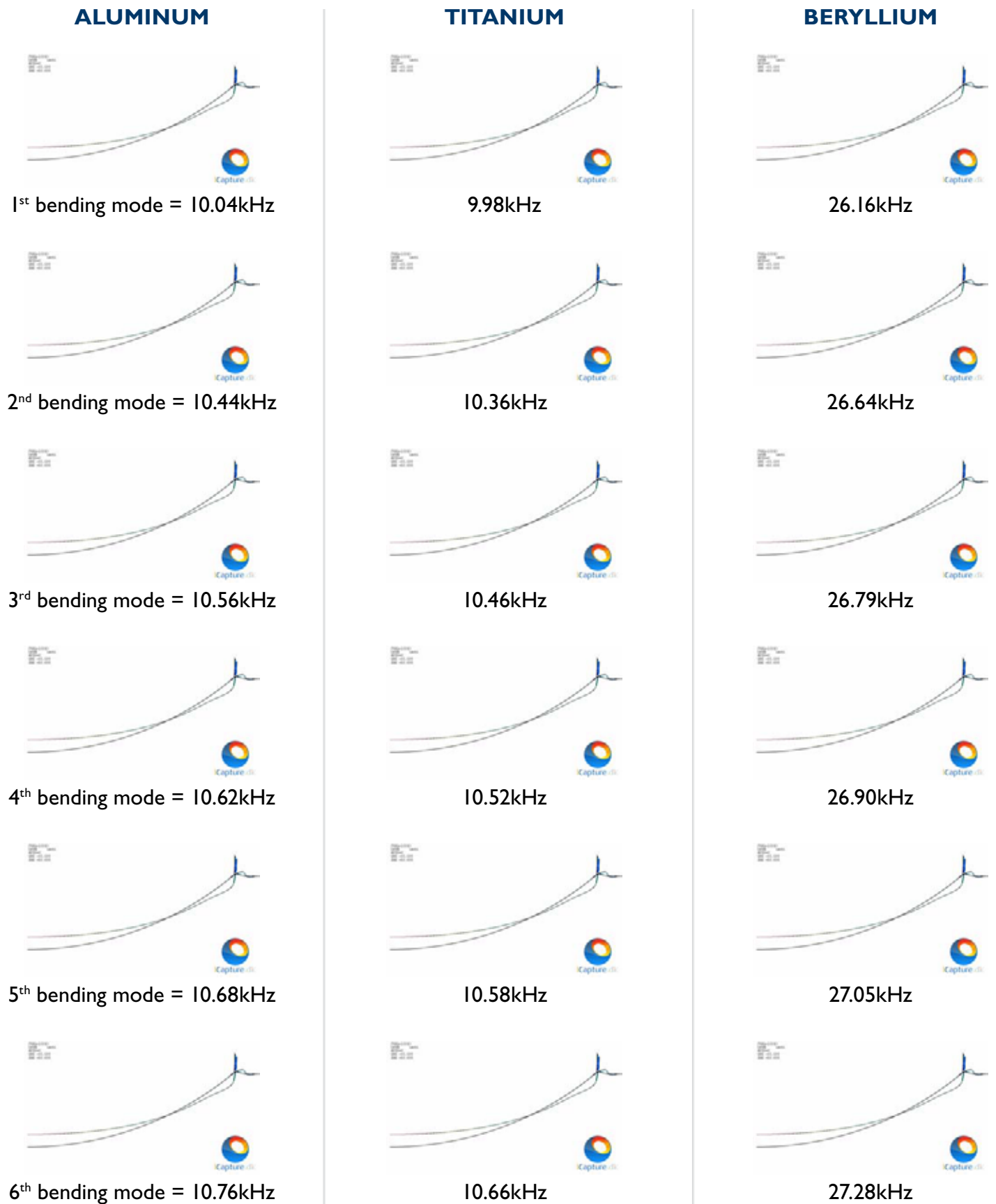
Figure 4. Bending Modes of 4" Compression Domes in Vacuo.
