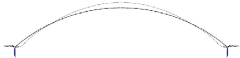
Figure 1. 2D Mode Shape at 1 st Bending Frequency of a Dome Diaphragm
