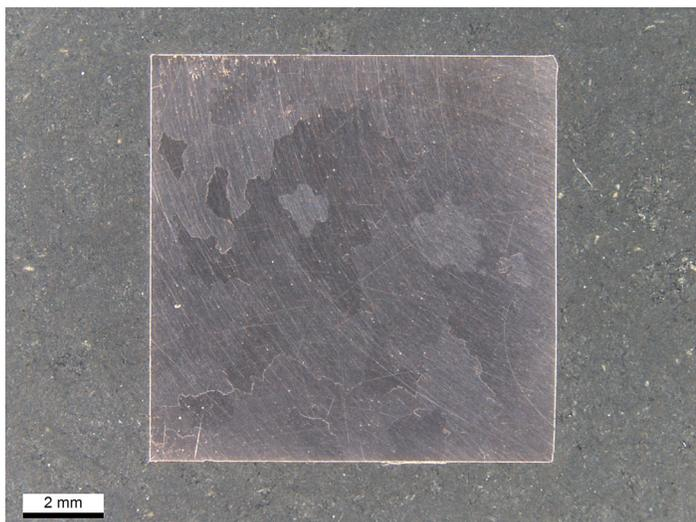
Macroscopic optical metallography shows the T2 CX90 alloy has a comparable cast grain size to that of the T3 CX105 alloy with no signs of large dendrites.
