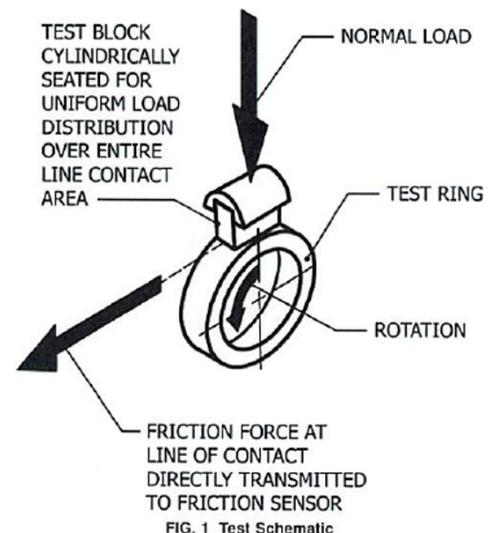
Test blocks were surface lapped (in the direction of sliding) to meet the surface finish requirements (4-8  $\mu\text{m}$ ) specified in ASTM G77.
