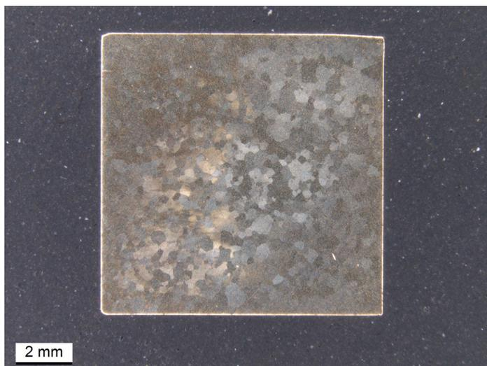
Macroscopic optical metallography shows the Mn Bronze alloy has considerably smaller cast grain size than the Materion alloys. This is due to the addition of Fe, which is a strong grain refiner. Limited dendrites or microsegregation is present due to small temperature window over which solidification occurs in this alloy.
