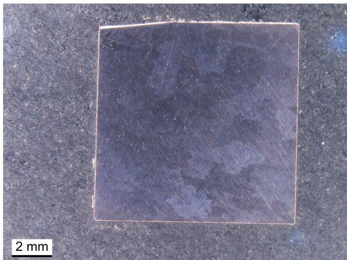
Macroscopic optical metallography shows the T3 CX105 alloy has a relatively large cast grain structure and no signs of large dendrites at this magnification.
