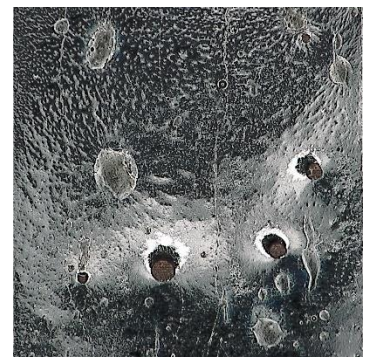
Figure 2: Failing dip test coupon
