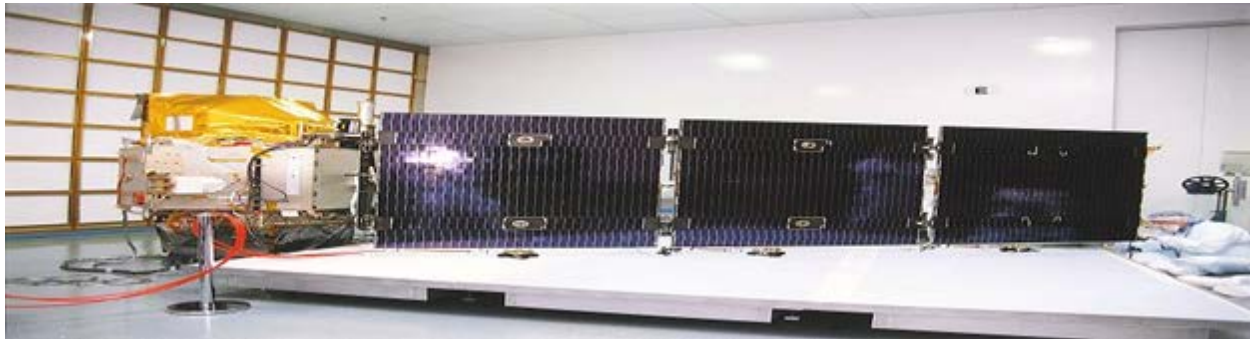
Figure 3. A solar panel “wing” made by Orbital ATK in its unfolded extent.
