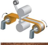
Materion Technical Materials' continuous clad process ensures stability and consistency throughout the coil. Cladding is done with a high percentage of cold reduction, and subsequent annealing steps ensure a true metallurgical bond between the Aluminum and the Copper alloy.
