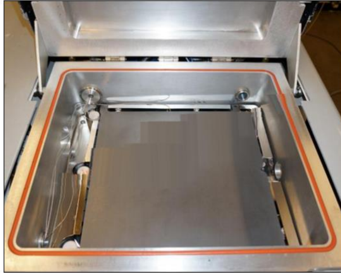
Illustration 14. Vacuum furnace inner chamber.
