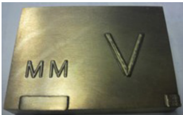
Figure 1: MoldMAX V Block Laser Welded with WeldPAK V Filler Metal.
