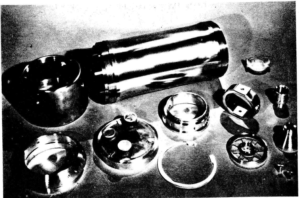
Figure 6- Beryllium copper components used in the underocean repeater housing.
