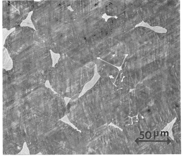
Figure 2 - C82500 alloy casting, solution annealed at 790°C (1450°F) and aged to peak hardness at 315°C (600°F) for 3 hr. Microstructure consists of Chinese script beryllides in a copper-rich solution matrix, with angular beta phase transformed to a lamellar aggregate of alpha and gamma phase. Striations are the result of metastable precipitation in the alloy. (Etchant 1, Table 1).
