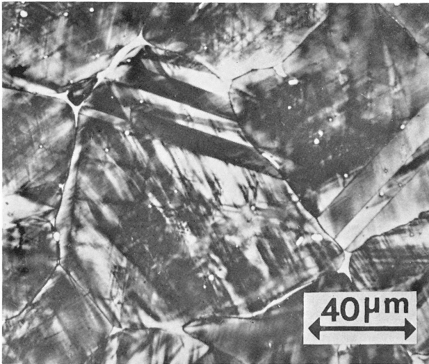
Figure 17 - C17200 alloy strip heated to 885°C (1625°F) and water quenched. The microstructure shows "burned metal" caused by solution annealing at too high a temperature. Incipient melting at the grain boundaries, caused by extreme temperature, resolidifies as beta phase. (Etchant 1, Table 1).
