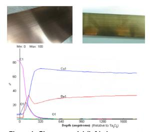
Figure I. Clean material (left) shown next to tarnished material. Below is an elemental profile of elements present in the tarnish versus depth in angstroms.
