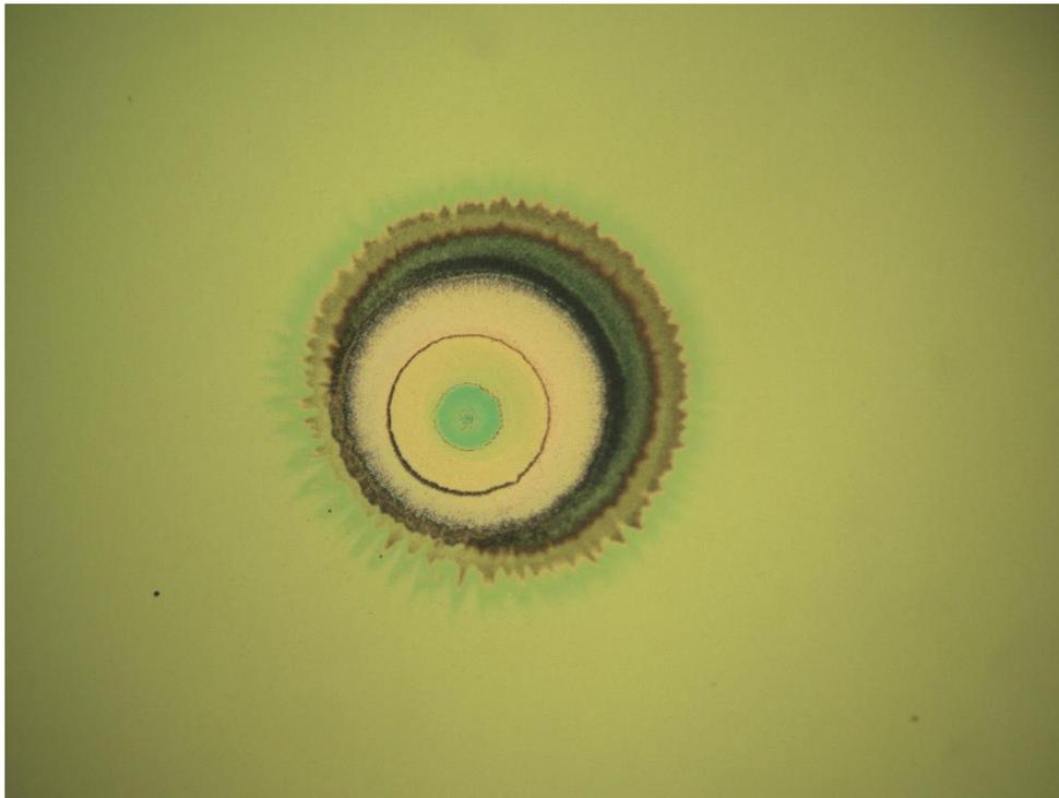
*Defect Driven Damage as seen on Samples From Laser Damage Competition.
