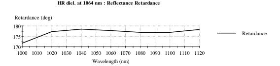
Figure 7. Retardance of a QW 1064 nm reflector with design  $(HL)^{12}$ .
