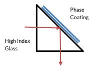
Figure 3. Configuration that produces controlled retardance at internal reflection.
