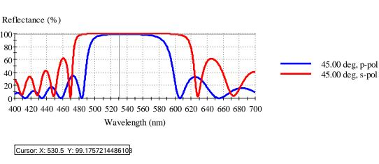
Figure 2. Reflectance at  $45^{\circ}$  AOI for the design (HL)<sup>12</sup>.
