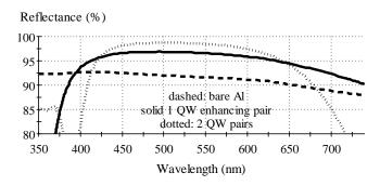
Figure 1. Al reflector protected by a single layer of SiO and enhanced by one and two QW pairs of TiO<sub>2</sub> and SiO<sub>2</sub>. Dielectric layers increase reflectance but narrow the wavelength coverage.
