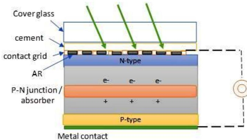
*Figure 1. Generic Silicon solar cell construction illustrating the separation of charges at the P-N junction.*
