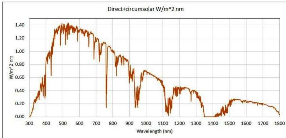
*Figure 3. Spectral insolation for AM 1.5. Integrated total is  $1.36 \text{ kW/m}^2$ . (ASTM G173-03 reference spectrum). Multi-junction cells respond to the energy between  $\sim 350$  nm and  $\sim 1600$  nm.*
