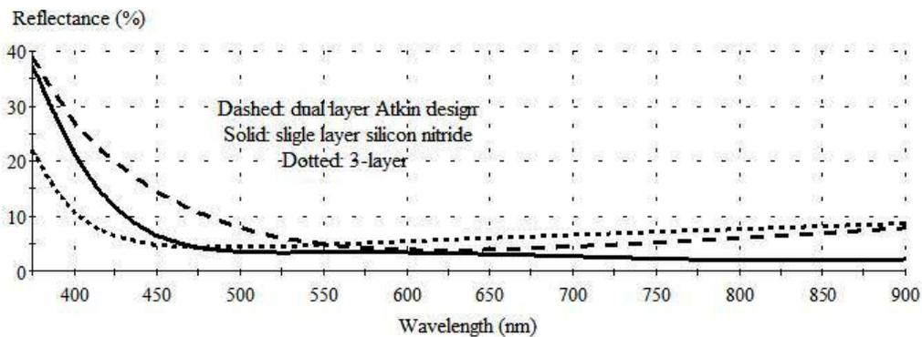
Figure 2. AR performances on a Silicon surface. Minimum values are 3-4%, and bandwidth varies with design.
