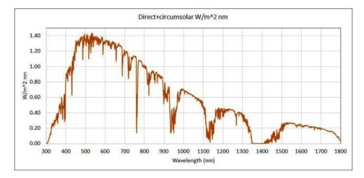
*Figure 3. Spectral insolation for AM 1.5. Integrated total is 1.36 kW/m<sup>2</sup>. (ASTM G173-03 reference spectrum). Multi-junction cells respond to the energy between ~350 nm and ~1600 nm.*
