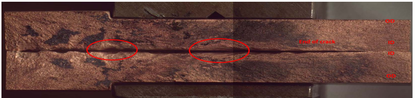
Figure 2: Fracture surface of the component, examples of divots circled in red
