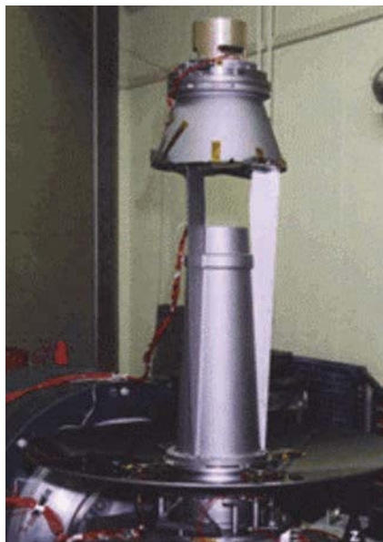
Fig. 5 — Prototype SIRTf telescope undergoing random vibration testing [5] .
