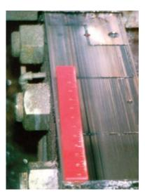
ToughMet® alloy ways provide better wear resistance & less friction as compared to aluminum bronze.
