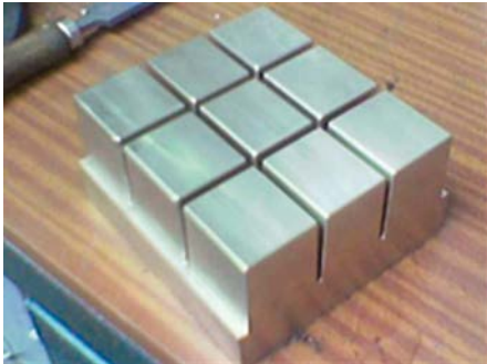
Example of one core insert used in the pallet container mold made of MoldMAX XL
