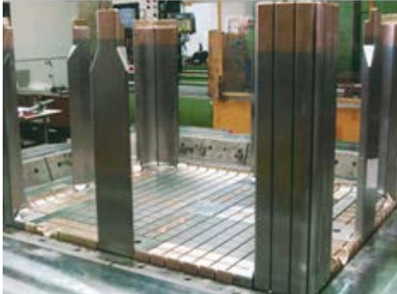
The old steel tool was replaced with MoldMAX XL due to its excellent machinability and balanced thermal conductivity engineered for large molds.
