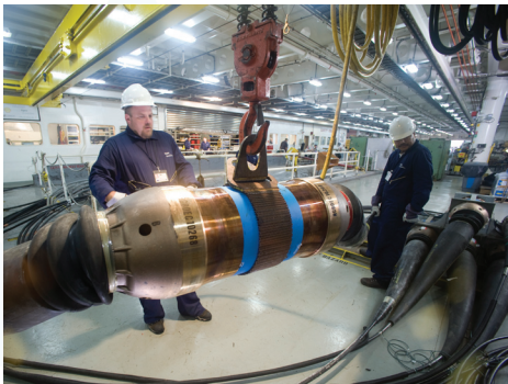
High strength undersea repeater housings made from copper beryllium alloys are packed with amplification equipment, loaded onto cable laying ships and deployed on the seabed.
