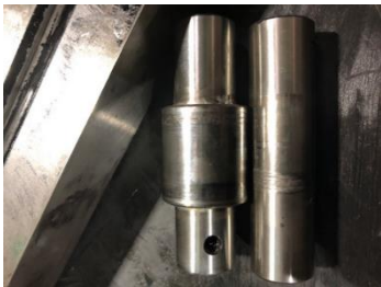
Steel-on-steel bushing and pin stuck together due to extreme galling.
